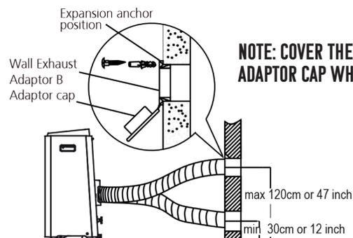
**NOTE: COVER THE HOLE USING THE ADAPTOR CAP WHEN NOT IN USE.**
