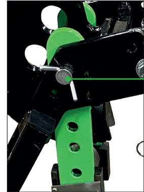
Remove the centre pin to allow the former disc to be put in place and then replace the centre pin to hold the former disc in position
