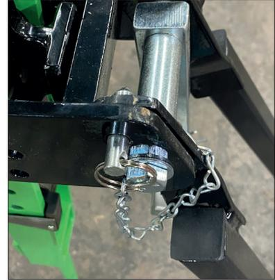
Insert the retaining pin to fix the A Frame in place.
