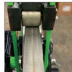
Turn the handle to lower the roller until it touches the top of the guide.
