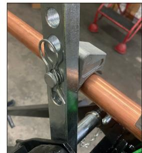
Insert the pipe under the tube stop and into the former disc
