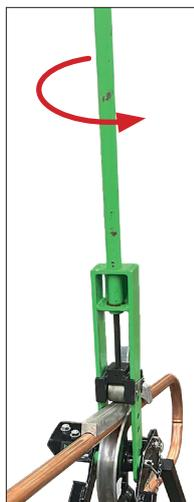
Turn the handle to lift the roller
